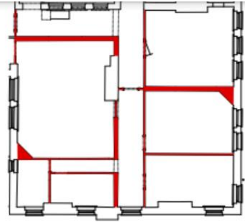
PROPOSED DEMOLITION PLAN
